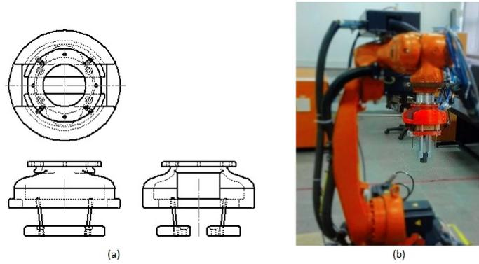
Figure 5: (a) Projection drawings of the final design (b) Final Prototype attached to a KUKA KR-5 robot for testing.
