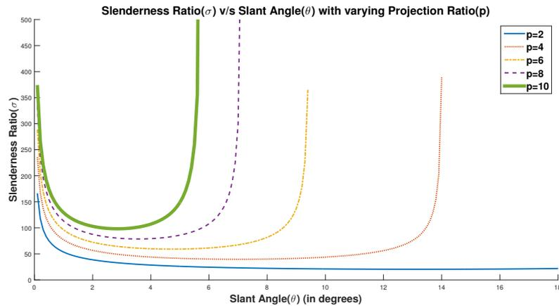
Figure 2: A dead band is observed in the plot. The range of the band increases with the decrease in the projection ratio.
