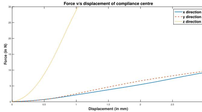
Figure 7: Force v/s displacement of compliant centre during experiment.
