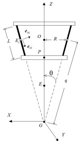
Figure 1: Geometry of the symmetrical beam arrangement design proposed by Ciblak & Lipkin [5]
