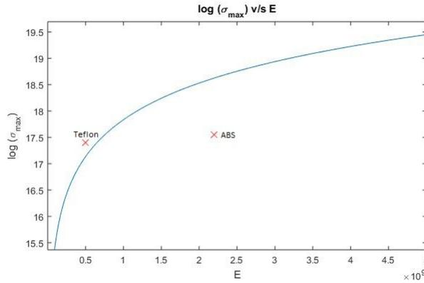
Figure 3: Graph between log of maximum stress and Young's Modulus. As the log of Teflon's Yield Strength lies above the log of maximal stress, Teflon beams are suitable for the design.
