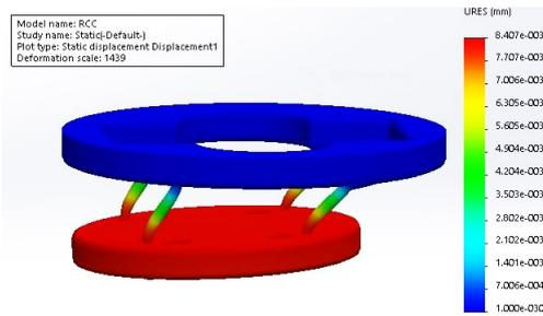
Figure 6: FE analysis of simplified version of final prototype. It was done to find the stiffness values in all six primary directions. Each value was found separately as the stiffness matrix had already been diagonalised.(Displacement scale magnification 1439)
